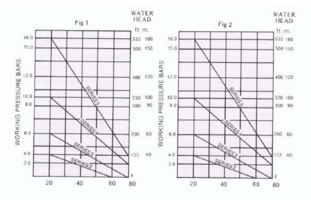
AMBIENT TEMPERATURE OF  $40^{\circ}$  C a Required working pressure of 6.0 bars Use 1 10 bar rated pipe.
