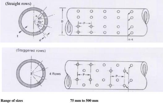
Longitudinal Pitch of wholes(LP) Hole Diameter Number of Rows **Angular Pitch of Holes**
