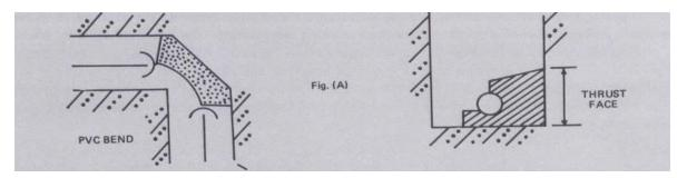
The design of uPVC pipes provides a safety factor of 2.1 after a life of 50 years at maximum working pressure. In designing thrust blocks it is logical to apply a similar factor of safety after calculating thrust forces on the maximum foreseeable line pressure.
