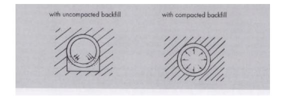
The ideal material should be free from large clay lumps (retained on a 3 in. sieve) from stones (retained on a 1 in. sieve) and sharp edged stones or flints, vegetable matter and from soil.
